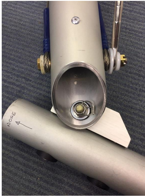
Fig 2: Note there is only one FW4-12 washer and that there are no washers between the cable thimbles and the tubing. Note also the upper rigging wire is fitted in the outer most rear position.
