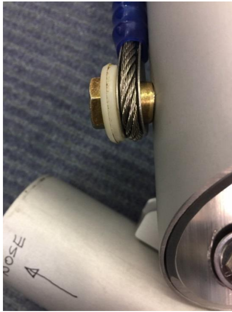
Fig 4: Shows the correct position of bush (Part No. 001-300) on the front lower rigging cable only. The purpose of the bush is to ensure equal tension in both lower side cables.
